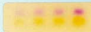
Red and orange dyes after electrophoresis. Differing volumes of the amplification reactions subjected to electrophoresis.
