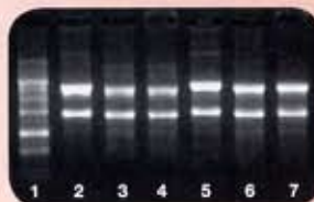
RNA extracted from ST6 cells and mouse tissue, using Bioline TRIsure and Competitor 1.
